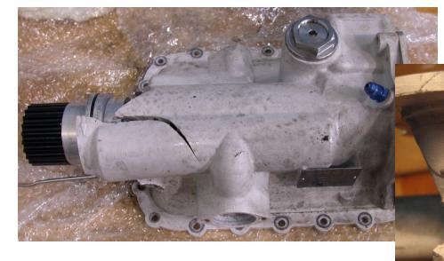
This pump blew after ingesting several screws Small FOD can cause big problems.
